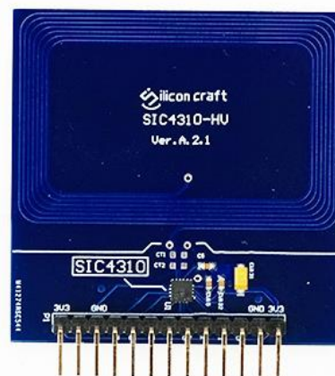
SIC4310-HV, An SIC4310 Demonstration Kit with UART Interface
