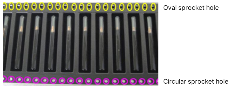
Figure 7-1: Product orientation and carrier tape dimension
