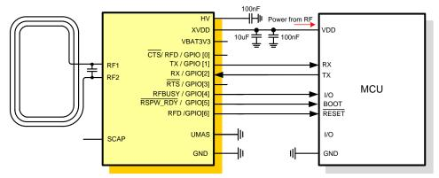
RF-powered configuration for firmware upgrade (Power harvesting)
